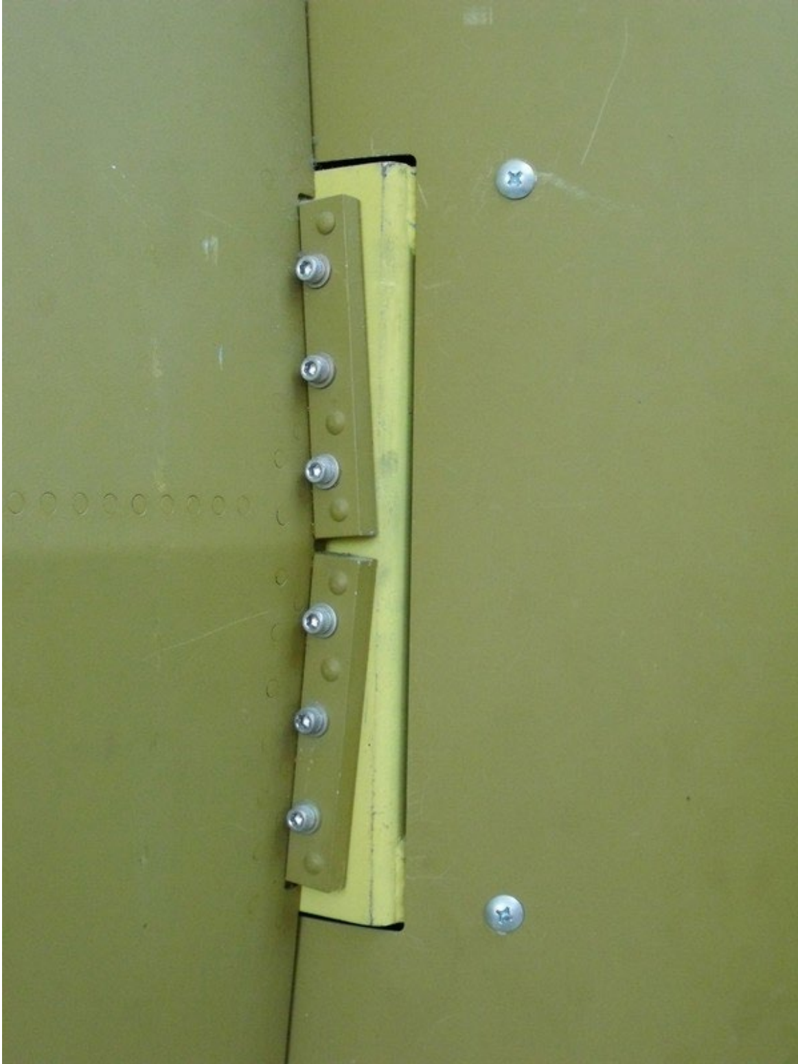
Photo 9: Nike Fin Root Rivet Detail
