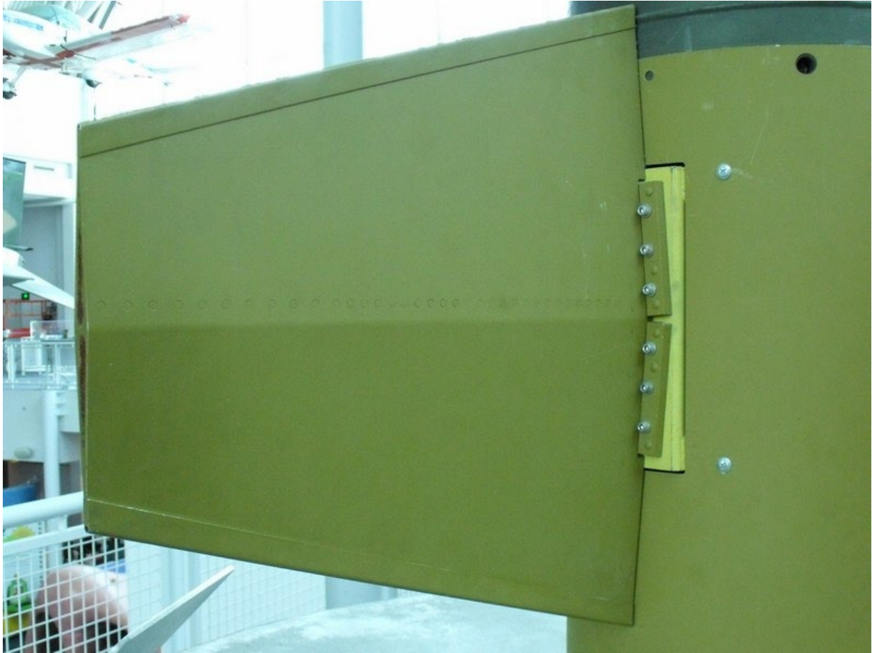
Photo 8: Standard Nike Fin Span Rivets
